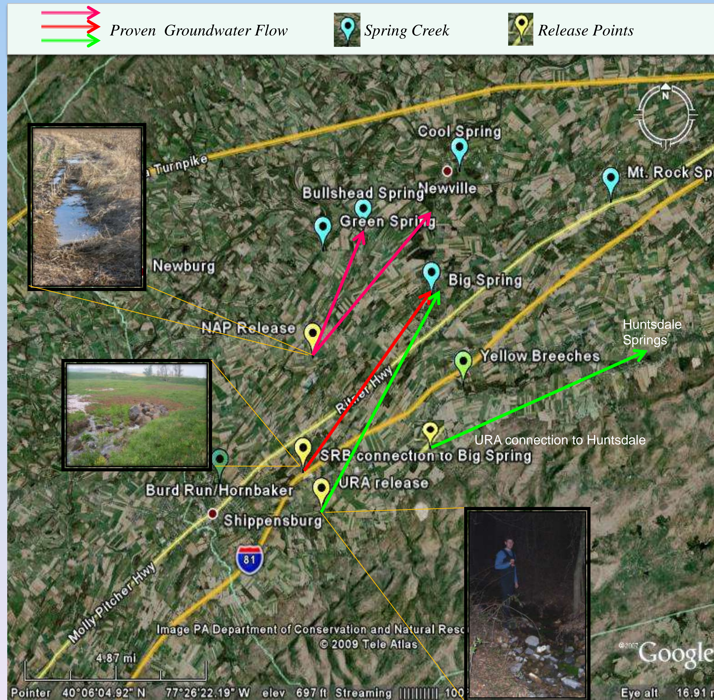
Figure 6 – Study springs, dye release locations, and proven connections in Western Cumberland County URA release - Thompson Creek near Cleversburg. NAP release is a sinking stream draining ag and possibly quarry runoff. SRB connection to Big Spring and URA to Huntsdale from Brookhart (2007).
